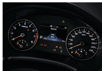
4.2英寸TFT LCD超级仪表盘
